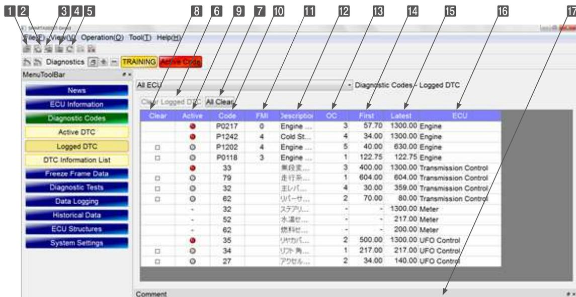
Figure 6-5 Logged DTC Screen
